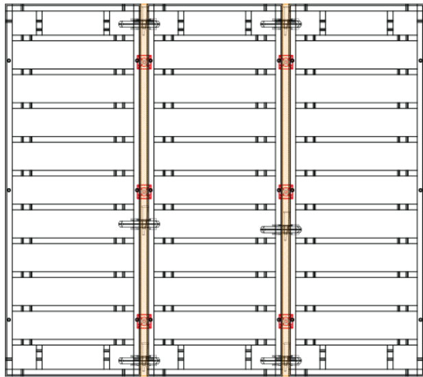
Couplers positioned away from cross profiles of panels
